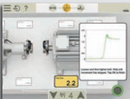
Soft Foot check on both machines
