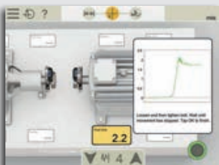
Soft Foot check on both machines
